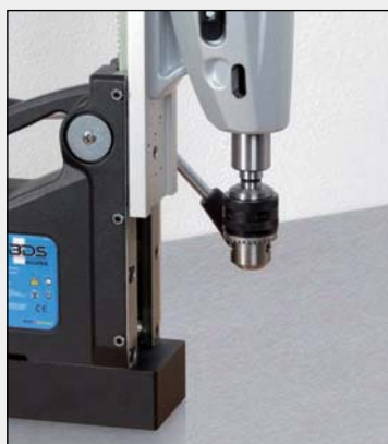
2. Place drill chuck in MT arbor.
