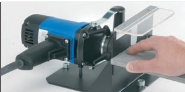
The optimum fixture for stationary deburring of small parts (Order No. ZKF 100)
