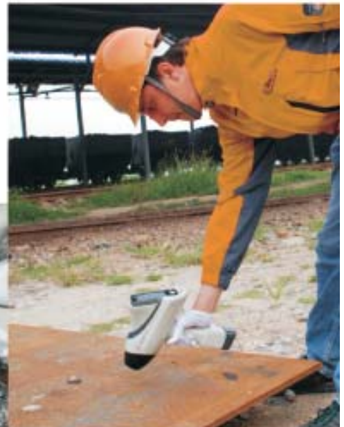
▲ Sorting of metals in sa vage station
